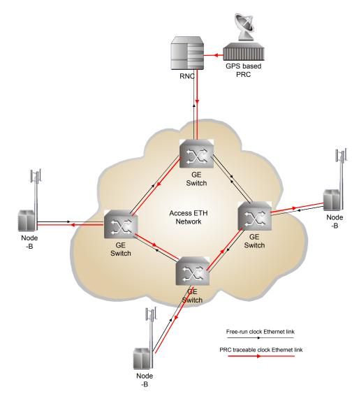
While such locking of the physical layer of Ethernet has doubtless been imagined before, the first attempt at its standardization as a network-wide solution is to be found in Clause 8.1.1 of the new ITU-T Recommendation G.8261. This standard mainly deals with timing aspects relating to transport of TDM over Ethernet networks, but while doing so explains how asynchronous Ethernet services may be mapped into a synchronous Ethernet network.
