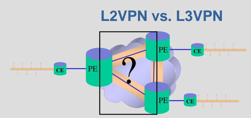
in L2VPN CEs appear to be connected by single L2 network PEs are transparent to L3 routing protocols CEs are routing peers
