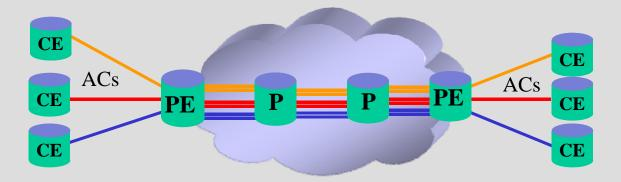
each customer network mapped to pair of (unidirectional) LSPs supports various AC technologies
