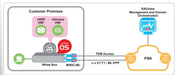
RAD's vAccess solution to this problem comprises several MiRIC-ML pluggable interfaces (transporting Ethernet or IP over TDM), the required device drivers, and a RAD-provided VNF to process the legacy MLPPP bonding protocol. Third-party VNFs, such as commercially available router software, can be chained after the vAccess VNF. The solution is depicted in the following figure. This vAccess solution has been successfully deployed by a tier-1 service provider.
