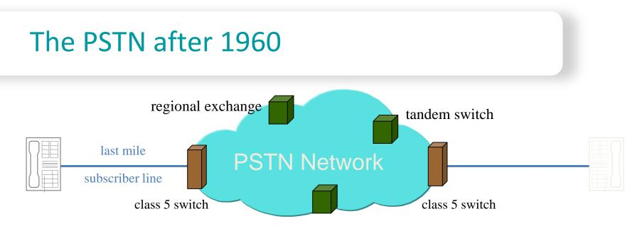
Analog voltages and copper wire used only in "last mile", but core designed to mimic original situation
