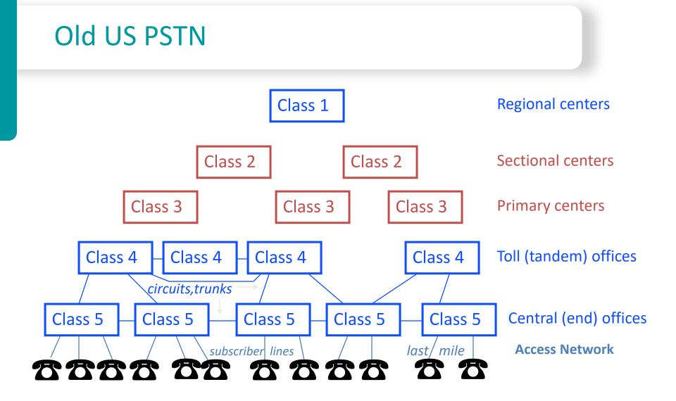
Class 5 switch is the sole interface to the subscriber lines Class 5 switches are interconnected but if no connection available Class 4 switches provide interconnection
