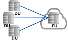
Using load-balancing/resilience techniques developed for cloud computing may allow a central site to service 100s of RRHs
