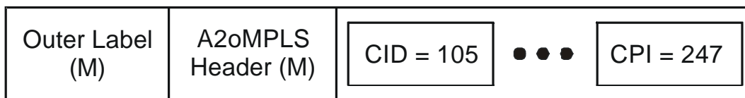
Figure 3-4 - Single-LSP structure for multiplexing CPS-Packets
