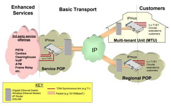
Building, Data or other Competitive Local Exchange Carriers or utility companies can increase their revenues by taking advantage of their wireless or optical data networks and use TDMoIP to extend T1 or E1 circuits between an entity and facilities at another location. In this way, the service provider can bundle private line services in addition to broadband data. Bundled services could include:
