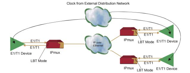
1) External master clock source provides out-of-band timing
